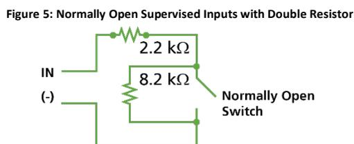
Normally Open Supervised inputs with two resistors must be connected with an 8.2K resistor in parallel and a 2.2K resistor in series to the input switch contacts.
