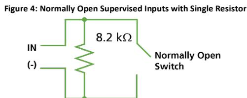
Normally Open Supervised inputs with one resistor must be connected with an 8.2K resistor in parallel to the input switch contacts.
