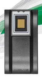
Rosslare's AYC-B7661 is a standalone biometric reader/controller. The AYC-B7661's sensor verifies between fingerprint data and a biometric template stored in the unit. The AYC-B7661 is convertible; it can work as a reader or as a standalone controller and supports 1:1 or 1:N technologies.
